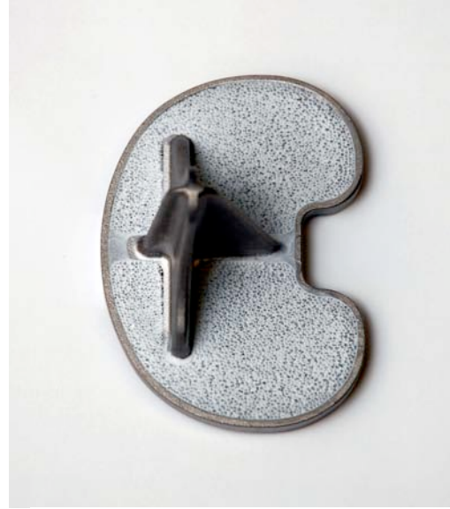
Figure 4. HA coating on tibia baseplate promotes bone integration.
